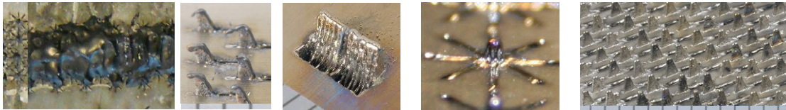
Fig. 1. (a) Rubber bonding onto metal stars; (b) Hooks; (c) Wall; (d) 8-leg star feature; (e) Array of single features.
