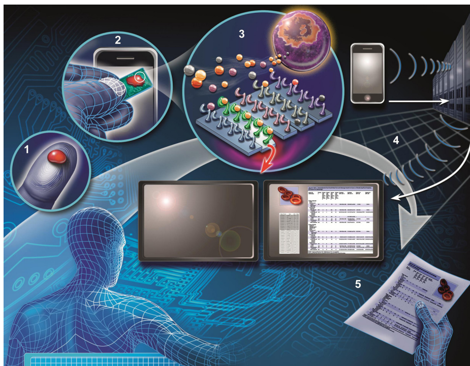
Fig. 2. Schematic diagram illustrating an example application of nanotechnology to medicine. (1) Home-based tests, (2) lab-on-a-chip technologies, and (3) cantilever technologies. An patient with inflammatory bowel disease (IBD) undergoing treatment could potentially use a smart phone to send the home-based test results to a server for processing (4), thereby reporting the inflammation marker level status to the patient's physician (5). Such techniques can potentially be used to adjust dosage towards treatment optimization.
