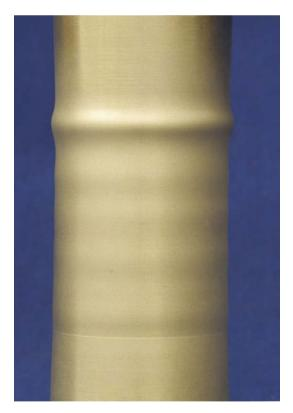
Fig. 9. Specimen CWR6 at the end of cycling showing wrinkles and localization at one end.
