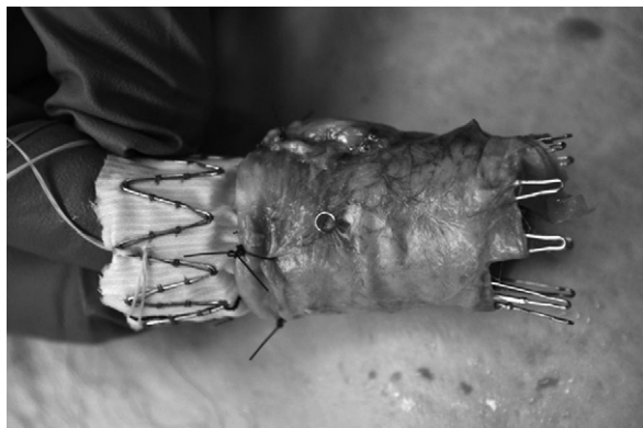
Fig 3. This Zenith endograft was reinforced with six EndoStaples before the application of displacement force (DF). The endograft was pulled out attached to the torn aortic tissue, proving the failure of the aortic tissue proximal to the fixation zone.
