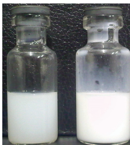
Figure 3. Picture of Rosmarinus officinalis emulsion (HLB 16.5) (left) and Illicium verum emulsion (HLB 16.7) (right) with droplet diameters of 91.12 nm and 246.6 nm, respectively.
