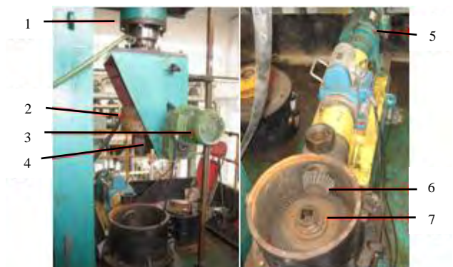
1—hydraulic cylinder for BP; 2—percussive drilling weight; 3—percussion electric motor; 4—boring bar slot; 5—rotating electric motor; 6—horizontal gear; 7—vertical gear
