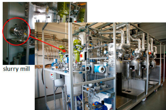
Figure 8. Illustration of continuous direct flue gas mineralization unit
