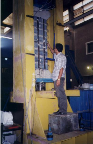
Figure 1. Test Set-up of rectangular columns under axial loads
