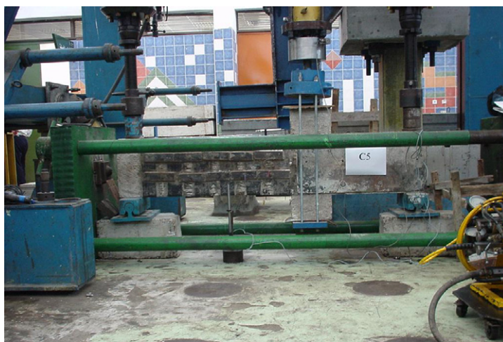
Figure 4. Test Set-up for rectangular columns tested under cyclic load
