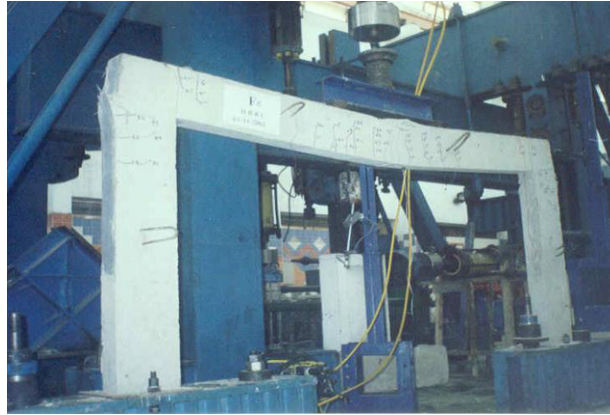
Figure 8. Test set-up of RC frames
