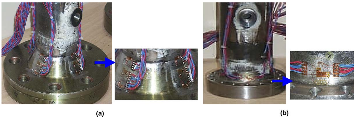
Fig. 2. Strain gauging at: (a) gasketed flange and (b) non-gasketed flange.
