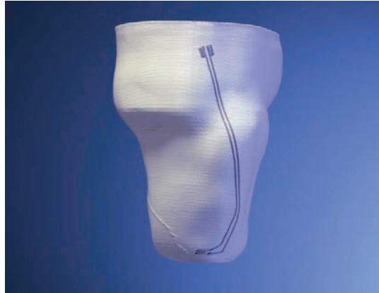
Fig. 5. Leg prosthesis part produced from PLA via FDM showing complex non-planar surfaces, with surface-integrated strain gauge sensors produced by Aerosol Jet™ printing and conductive paths deposited via micro-dispensing, both using the modular manufacturing platform [74].
