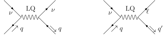
Fig. 1. Resonance processes via a leptoquark LQ in the UHE neutrino nucleon scattering. Left: the neutral current events. Right: the charged current events. The case of interest is a \tau -neutrino and a \tau -lepton.
