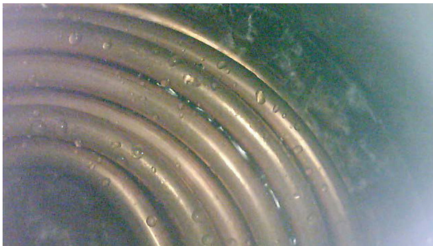
Fig. 7. Droplets on the evaporation/condensing heat exchanger
