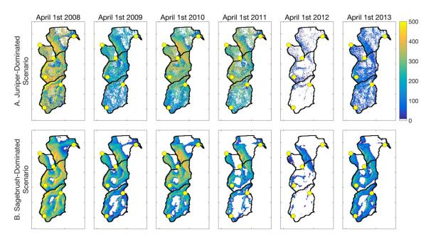
**Figure 8.** Modeled snow water equivalent (mm of SWE) distributions on 1 April of each water year for the **A,** juniper-dominated scenario and **B,** sagebrush-dominated scenario. Late season differences show that the sagebrush-dominated scenario results in more SWE stored in drifts opposed to the juniper-dominated scenario, which results in a more even snow distribution. Yellow circles indicate the location of weather stations.
