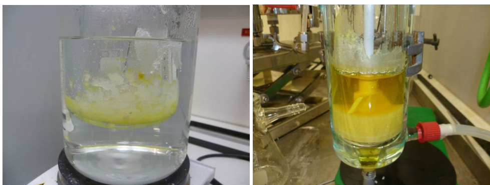
Fig. 1. Recrystallization of \text{Na}_2\text{S}\cdot 5\text{H}_2\text{O} . Left: melting/dissolving of feed material; right: yellow mother liquor with white crystals
