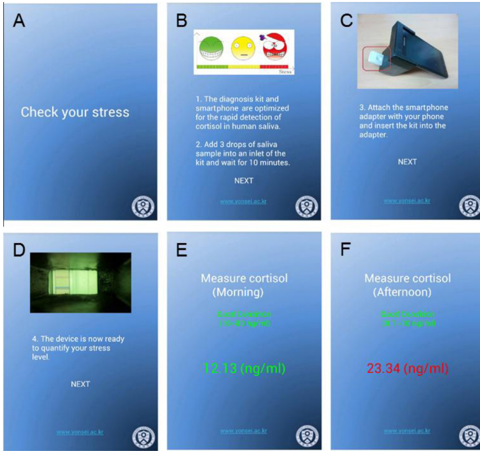
Fig. 2. Screenshots of our application running on an Android smartphone. (A) Once the application runs (B–D) the user reads the testing protocol explained under the pictures. (E and F) Following the activation of the smartphone camera, the user can simply touch the screen to capture the images of the test line. The acquired images are rapidly processed on the smartphone to quantify the cortisol amount within the human saliva sample.
