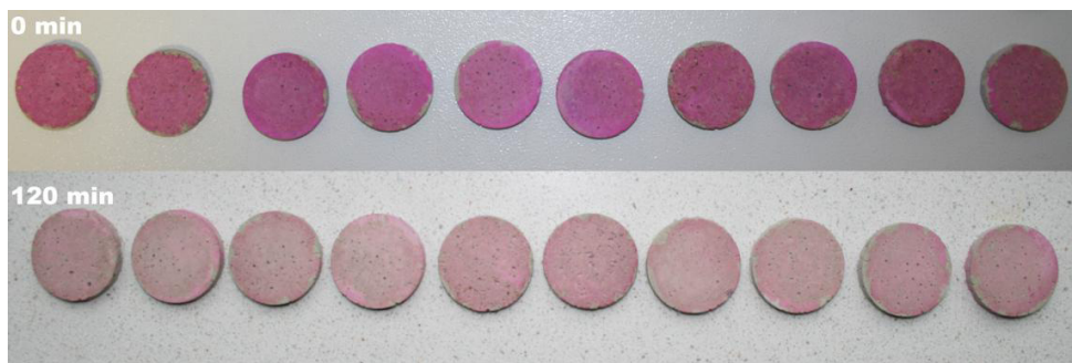
Fig. 3. Discoloration of rhodamine B on the surfaces of tested mortars after 0 min and 120 min of UV light irradiation.
