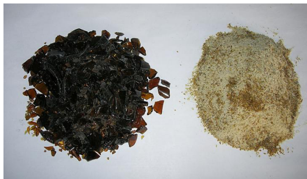
Fig. 1. Photograph of obtained waste glass (left) and after milling process (right) with particles size less than 2 mm.
