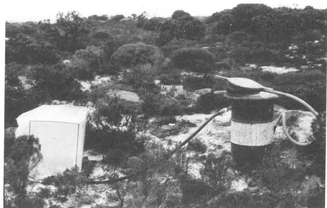
Figure 1 Apparatus used to pump smoke from burning fynbos plant material in a drum into plastic tents placed onto natural A. capitata seed banks in the unburned Olifantsbos population.
