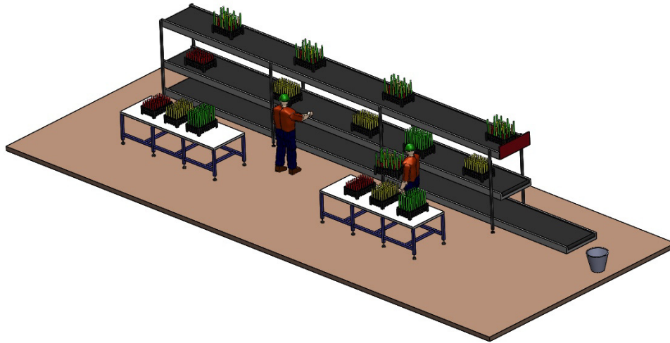
Fig. 5. Schematic representation of the redesigned plant production line
