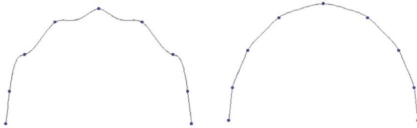
Fig. 3. Ordinary interpolating curve (left) and our shape preserving interpolating curve (right) for scattered data (B).
