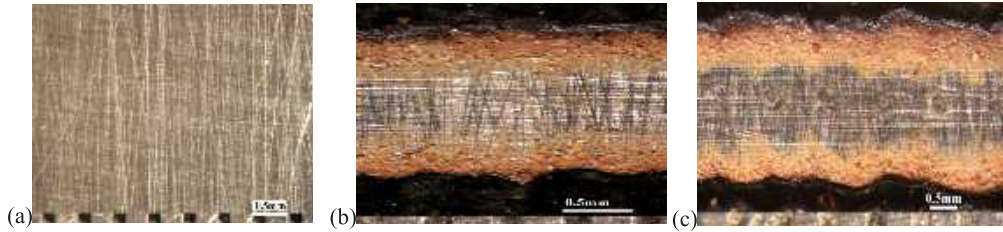
Fig. 2. Photographs of stainless steel samples (a) bare base metal, (b) complete removal of paint by the water-jet assisted laser beam, laser peak power = 1800 W, modulation frequency = 200 Hz, duty cycle = 10%, and scan speed = 7000 mm/min; (c) onset of melting in the central zone, scan speed = 6000 mm/min, other conditions same as (b).
