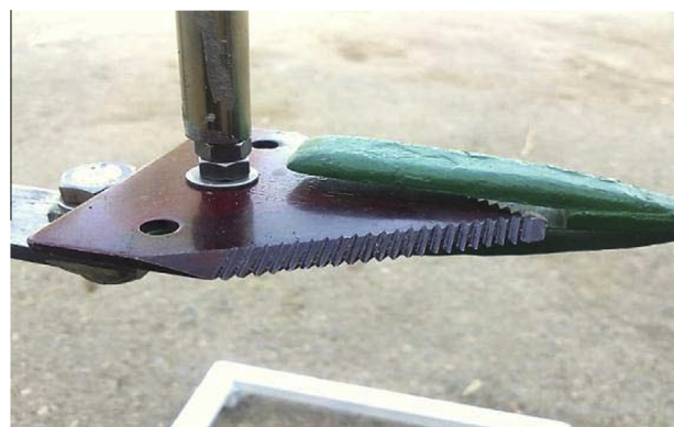
Figure 8 Blade and finger statue during impact cutting.
