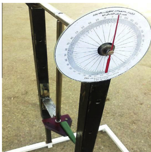
Figure 7 Pendulum impact system.
