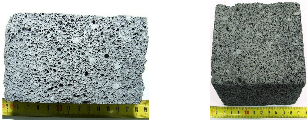
Fig. 2. The exemplary surface of the obtained geopolymer foams (sample F4).
