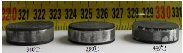
Fig. 2. Morphologies of the three-layer foamable composites obtained at different temperature under hot-dipping alloy: Zn-5wt.%Al, axial pressure: 6MPa, holding time: 90min
