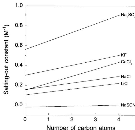
FIGURE 4 Linear dependence of the salting-out constant  $k_s$  (see Eq. 1) on the number of side-chain carbon atoms in the blocked amino acids studied by Nandi and Robinson (1972a) (see Fig. 3). The figure has been redrawn.
