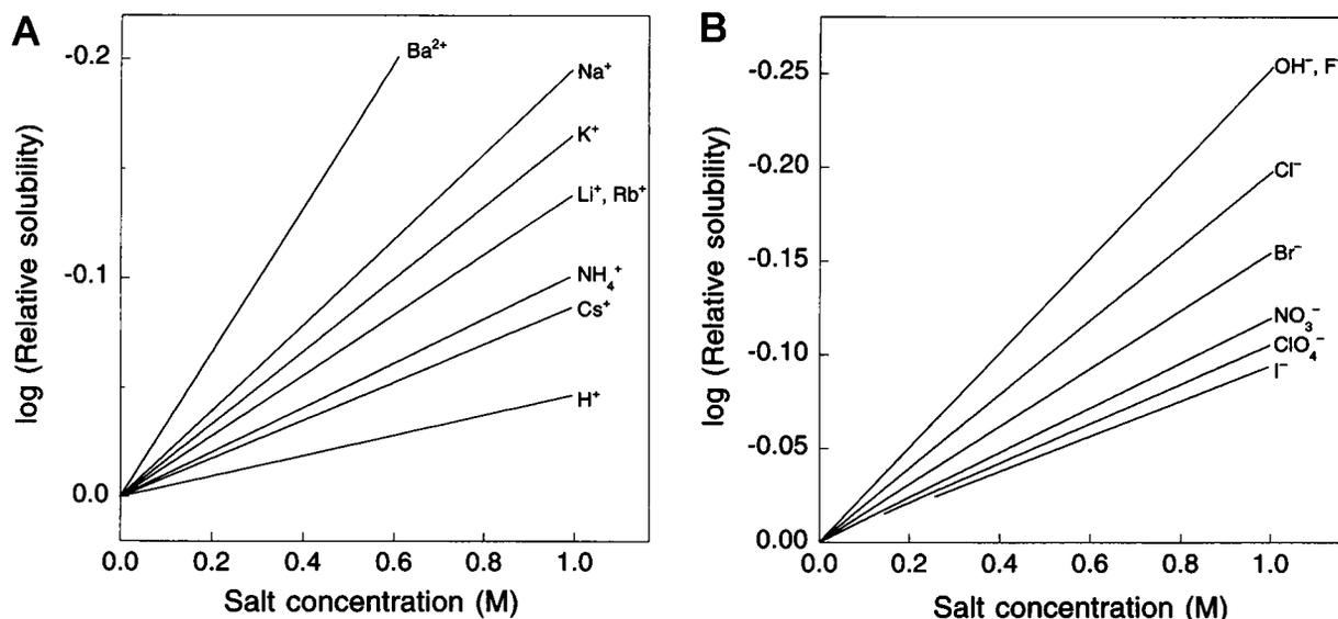
FIGURE 1 Effectiveness of various Hofmeister ions in salting out benzene from aqueous solution. The results are plotted according to the Setchenow equation, which tests if the data fit the weak interaction model. (A) Cations (chloride salts); (B) Anions (sodium salts). The data are from McDevit and Long (1952); the figure has been redrawn. Relative solubility refers to the ratio of benzene solubilities in the presence of salt (at the concentration indicated) and in the absence of salt.
