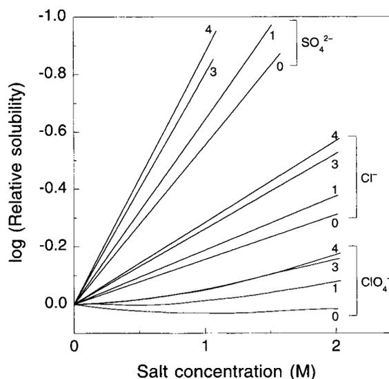
FIGURE 3 Comparison between the effectiveness of  $\text{Na}_2\text{SO}_4$ ,  $\text{NaCl}$ , and  $\text{NaClO}_4$  in salting out at 25°C blocked amino acids containing straight-chain aliphatic side chains with 0, 1, 3, or 4 carbon atoms. Data are from Nandi and Robinson (1972a); the figure has been redrawn.
