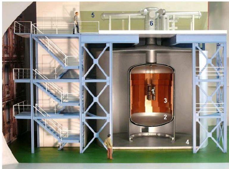
Fig. 1. Model of the GERDA experiment. The labels are: 1 = detector array (not to scale), 2 = cryostat, 3 = inner copper lining, 4 = water tank, 5 = clean room, 6 = lock for Ge detector insertion.
