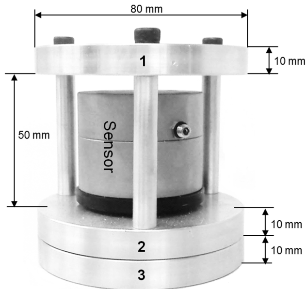
Figure 1. View of 'caged' accelerometer
