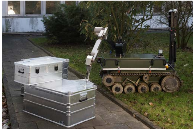
Fig. 1. Taking samples in a possibly contaminated area is a typical application for tele-operated mobile manipulation.
