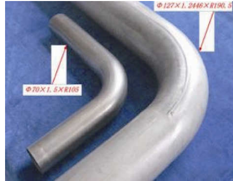
Fig. 5 Experimental bent tubes with large diameter.
