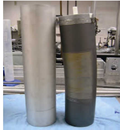
Fig. 9 Laser bending of large-diameter thin-walled tube [80].
