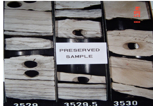
Fig.2b Samples from the Bahariya Formation (left) side laminated and non-laminated (right).
