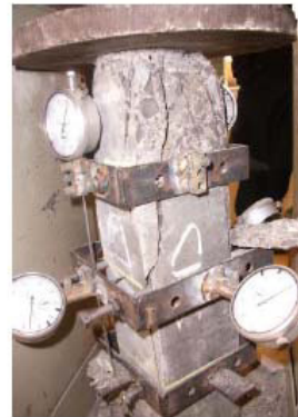
Figure 3: Deformations measured on the test-tube during compression
