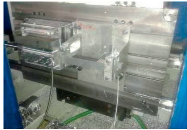
Fig. 3 Residual stresses measurement system for a conventional CNC machine
