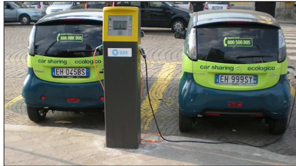
Fig. 2. An example of recharging station for one of the electric car sharing of Milano ( www.car-sharing-evai.it ).
