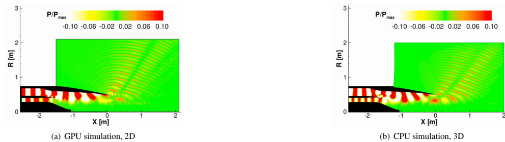
Figure 7: Instantaneous pressure contours obtained using isentropic models
