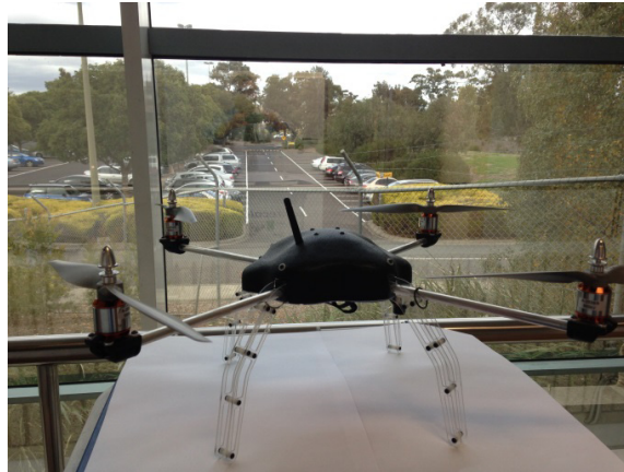
Fig. 9. A quadrotor for the power line inspection investigations.
