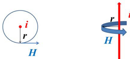
Fig. 2. (a) Current, i , radius, r , and Magnetic field, H , vectors. (b) Ampere’s Law known as Right Hand Rule.
