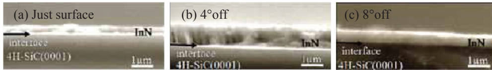
Fig. 5. Cross-sectional SEM images of InN on 4H-SiC (0001): (a) 0° (just surface), (b) 4° and (c) 8° off-angles
