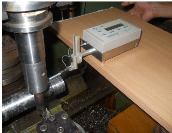
Fig. 8. Measuring the surface roughness of the workpiece using ‘TALYSURF’ equipment.
