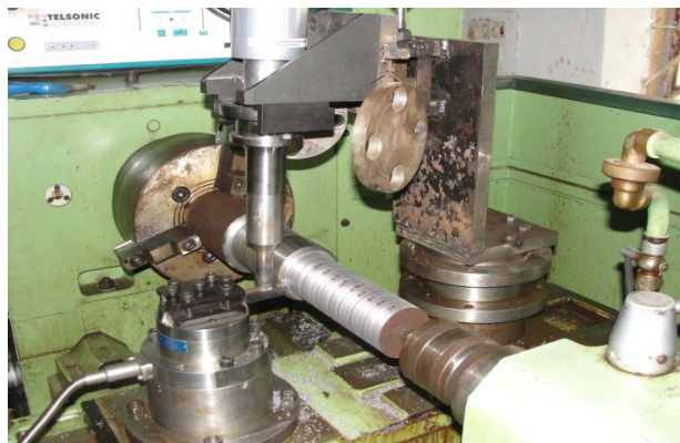
Fig. 6. Work piece preparation in UAT using lathe (HMT Model NH 26).
