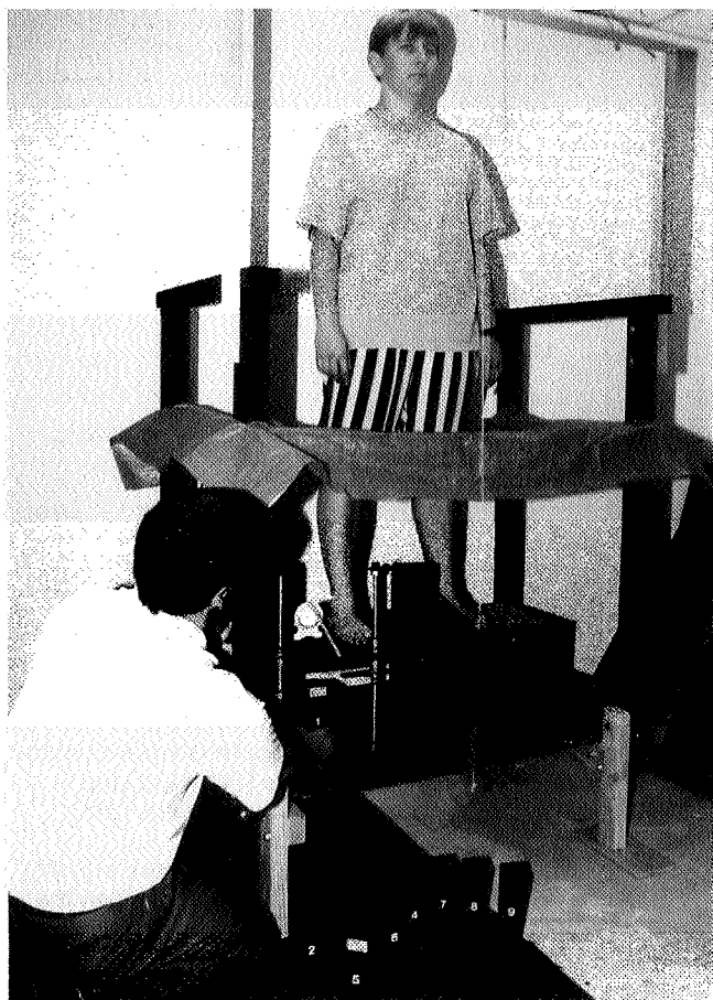
Figure 1. A subject standing on the purpose built ankle movement extent discrimination apparatus, AMEDA.
