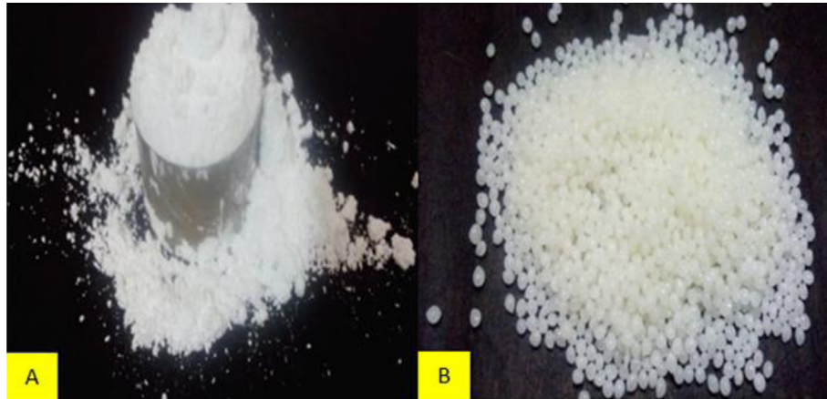
Fig. 3. Used additives appearance and physical state (A) Zeolite (B) Sasobit.
