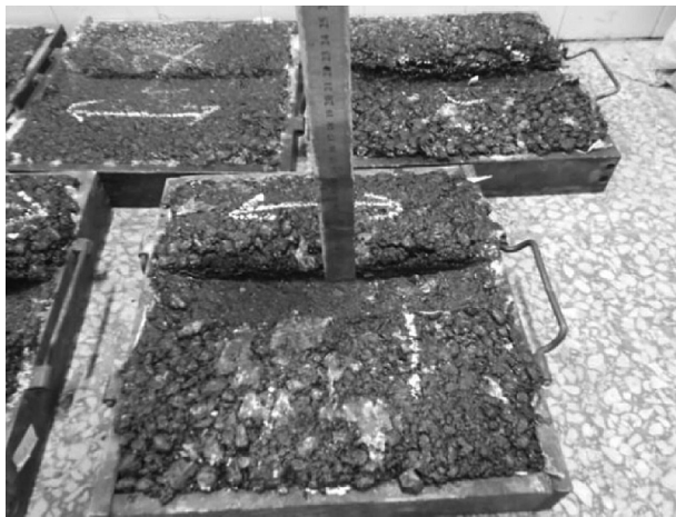
Fig. 6 – Failed rutting test (initial phase).
