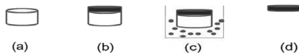
Fig.1 Route chart for preparation of free-standing coatings: (a) polishing of carbon steel substrate; (b) preparation of the single 7YSZ coatings; (c) erosion in a hydrochloric acid solution; (d) cleanness for the final free-standing coatings
