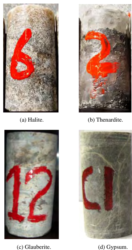
Fig. 1 Samples of four lithologies in bedded salt deposits.
