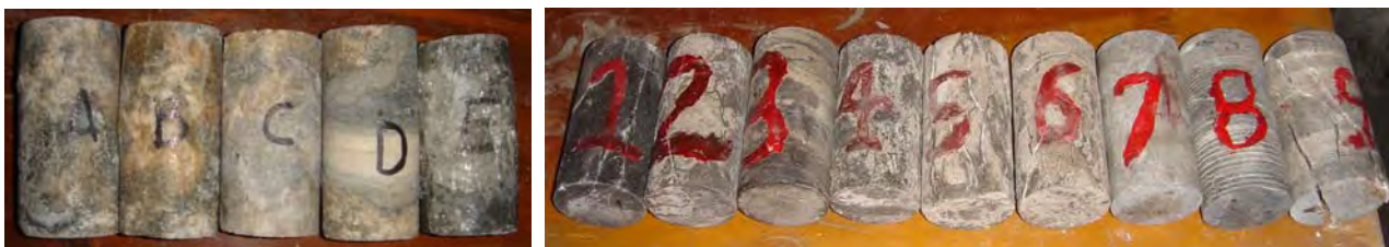
(a) Specimens of thenardite and halite after failure.
