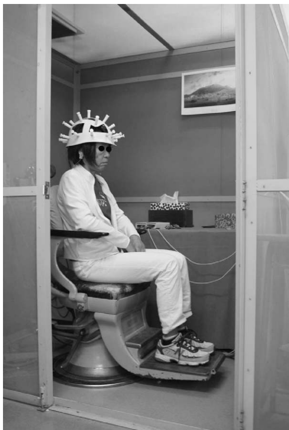
Figure 1 Electroencephalographic (EEG) measurement in a semi-anechoic room. Measurements were performed while the subjects were seated in a resting position with their eyes closed.
