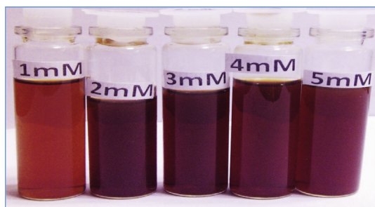
Fig. 1 – Digital optical images of synthesized silver nanoparticles with different conc (1–5 mM) of \text{AgNO}_3 .
