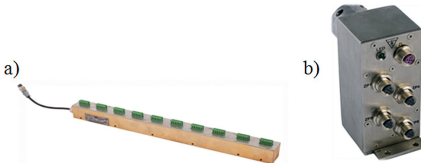
Photo 2 – The device designed to control and gather data a) LR-01/10/CH b) BP-01/4/T.
