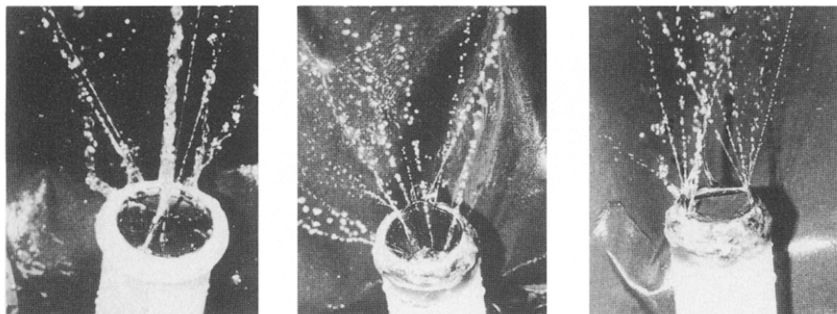
Figure 5. Closeup photographs of prosthetic valves mounted on a water-filled tube in the reverse position; a seal was obtained with silicone rubber. The retrograde perfusion pressure was 74 mm Hg; the orientation is as in Figures 3, 4 and 6. Left, Tilting disc prosthesis. A central jet issuing from the central hole in the disc is surrounded by smaller jets emerging from the disc circumference. Center, Bileaflet prosthesis. The closure line of the leaflets runs into the plane of the picture; multiple jets emerge from the leaflet hinge points and appear predominantly to diverge from this perspective. There is also minor regurgitation at the circumference of the leaflets and from the central closure line. Right, Bileaflet prosthesis. The closure line of the leaflets runs horizontally in the plane of the figure. Viewed from this vantage, the many jets emerging from the leaflet hinge points appear predominantly to converge.
