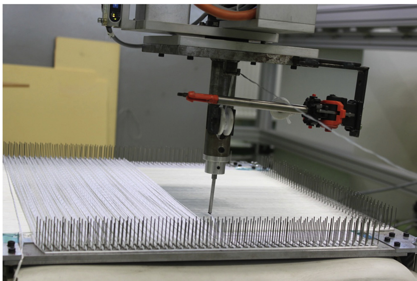
Fig. 4. Glass fibre placement for a [0, 90]_7 configuration at the Manchester tow placement machine [50].
