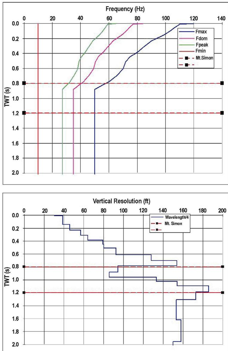
Figure 3: Analysis of bandwidth of 2D data and vertical resolution. a) Frequency content against depth. b) Variation in thin bed resolution with depth; vertical resolution is a function of the maximum interpretable frequency and velocity.
