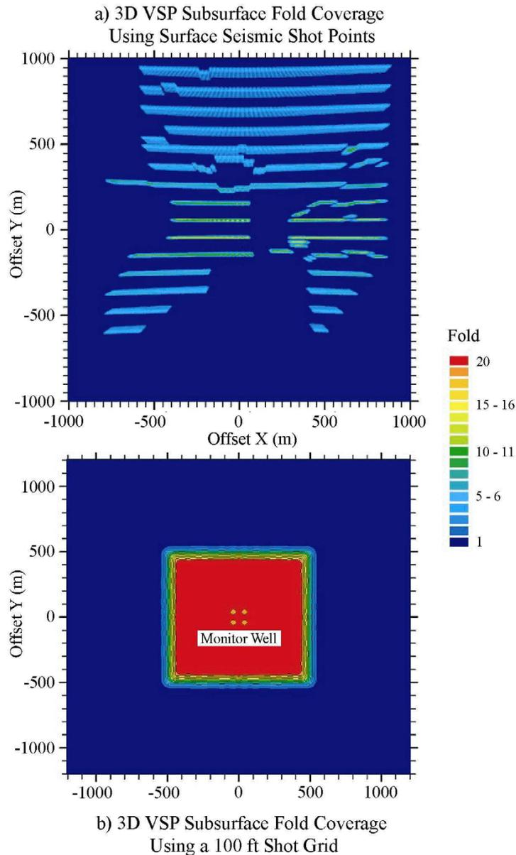
Figure 6: 3D VSP fold coverage modeling. a) The subsurface fold coverage obtained using the 3D surface seismic shot points. The shot points and shot lines result in 2D walkaway VSP images rather than 3D VSP images. b) 3D VSP fold coverage using a 100 ft shot grid.
