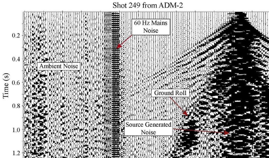
Figure 5: Example of the noise recorded in a shot gather at the north end of the north-south 2D line. Types of noise include ambient noise in the area, electrical noise from power lines, ground roll, and source generated noise. This is one of the shots farthest from the plant and is relatively quiet. Trace spacing is 110 ft.
