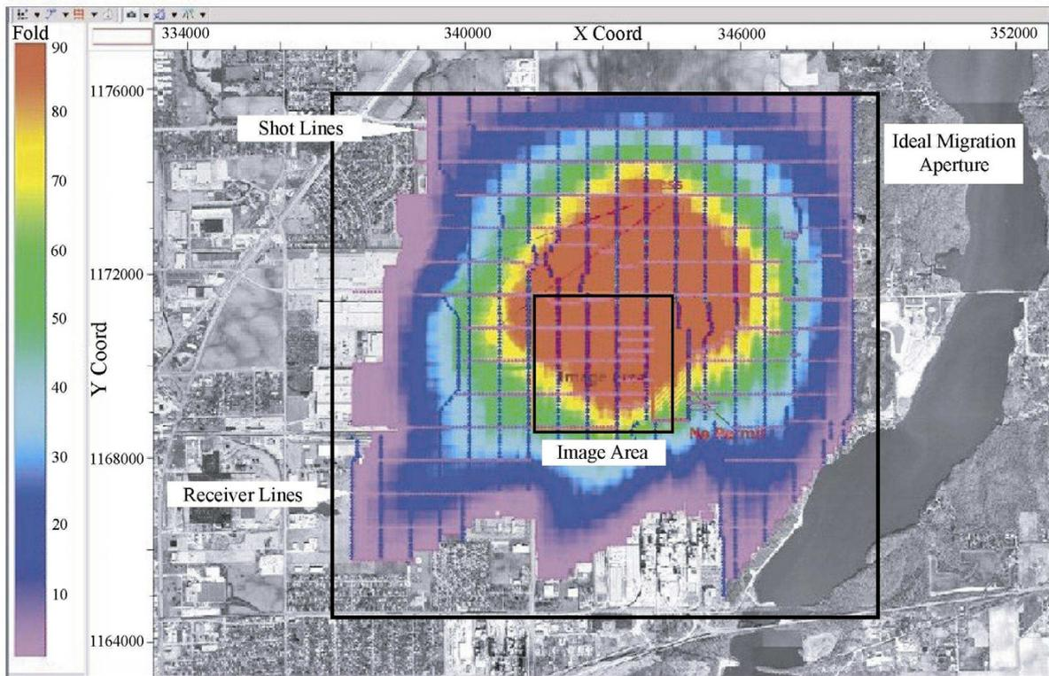
Figure 4: The best case source – receiver lay-out and fold coverage for the ADM site given surrounding surface constraints. Source lines are in purple, and receiver lines are in blue. Fold coverage is based on a 40 x 40 ft bin size. The ideal migration aperture and subsurface image area are highlighted in black.
