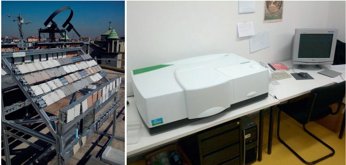
Fig. 3. (a) Test facility sample holder with several samples with different tilt angles and (b) UV/Vis/NIR Spectrophotometer PerkinElmer Lambda 950.
