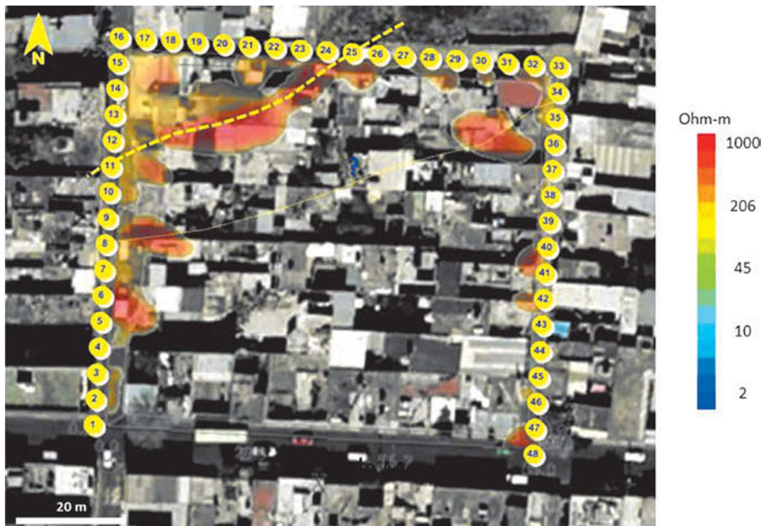
Figure 9. The working cube is observed from the top. The Google image (Google, 2012) is superimposed on top of the resistivity anomalies. Observe the fracture in the NE-SW direction.
