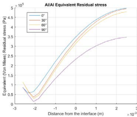
Figure 5: Through-thickness equivalent residual stress profiles for Al layers deposited on Al substrate.
